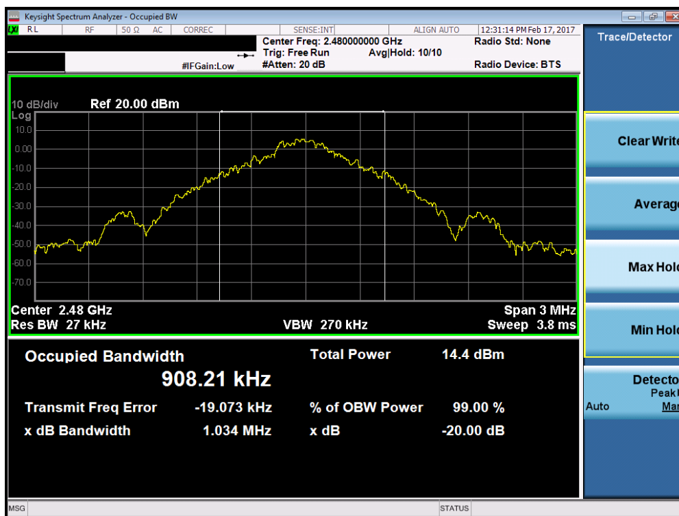
Plot 7-3. 20dB Bandwidth Plot (Bluetooth, 1Mbps – Ch. 78)
