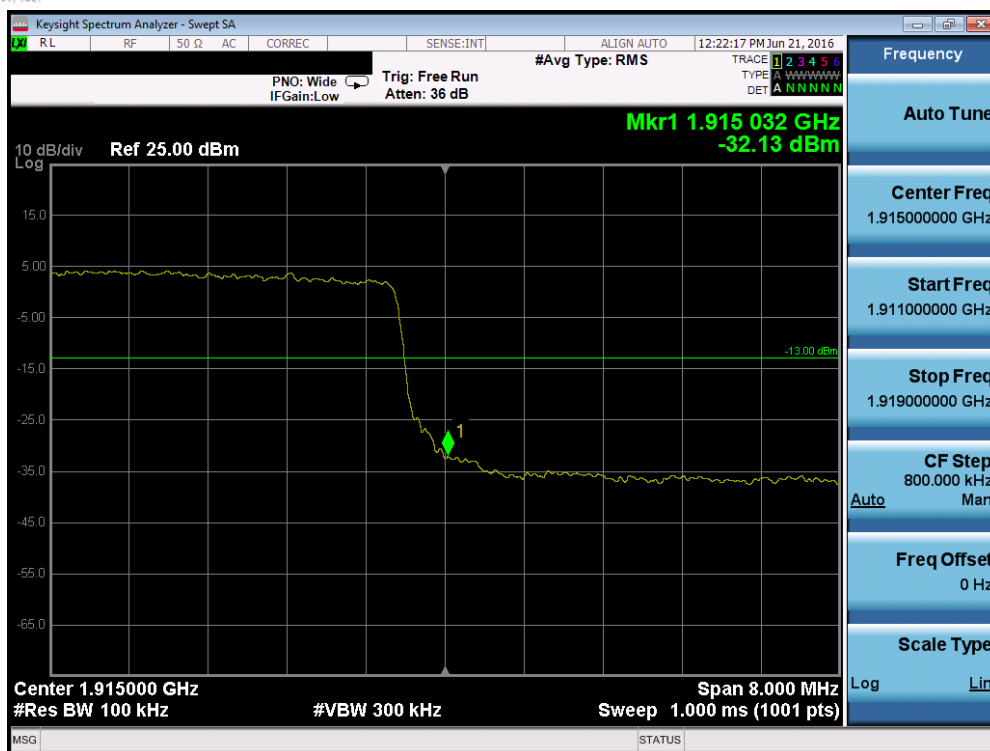
Plot 7-147. Upper Band Edge Plot (Band 2/25 – 10.0MHz QPSK – RB Size 50)
