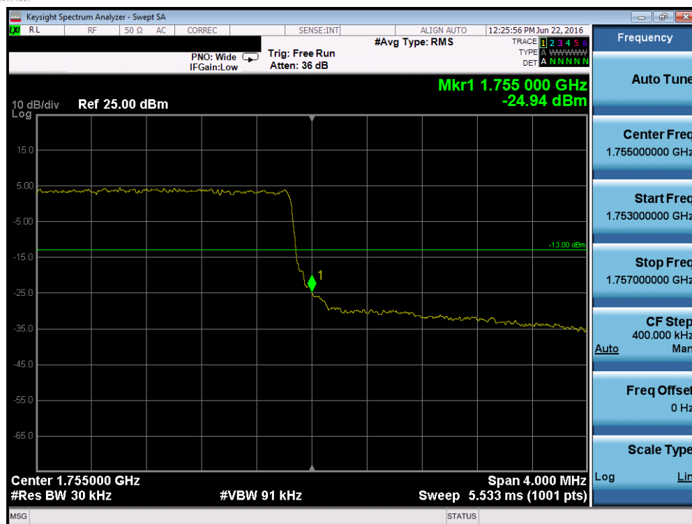
Plot 7-115. Upper Band Edge Plot (Band 4 – 3.0MHz QPSK – RB Size 15)
