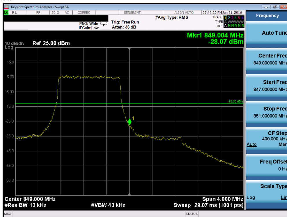
Plot 7-95. Upper Band Edge Plot (Band 5/26 – 1.4MHz QPSK – RB Size 6)
