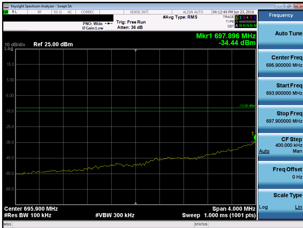
Plot 7-80. Lower Extended Band Edge Plot (Band 12 – 1.4MHz QPSK – RB Size 6)
