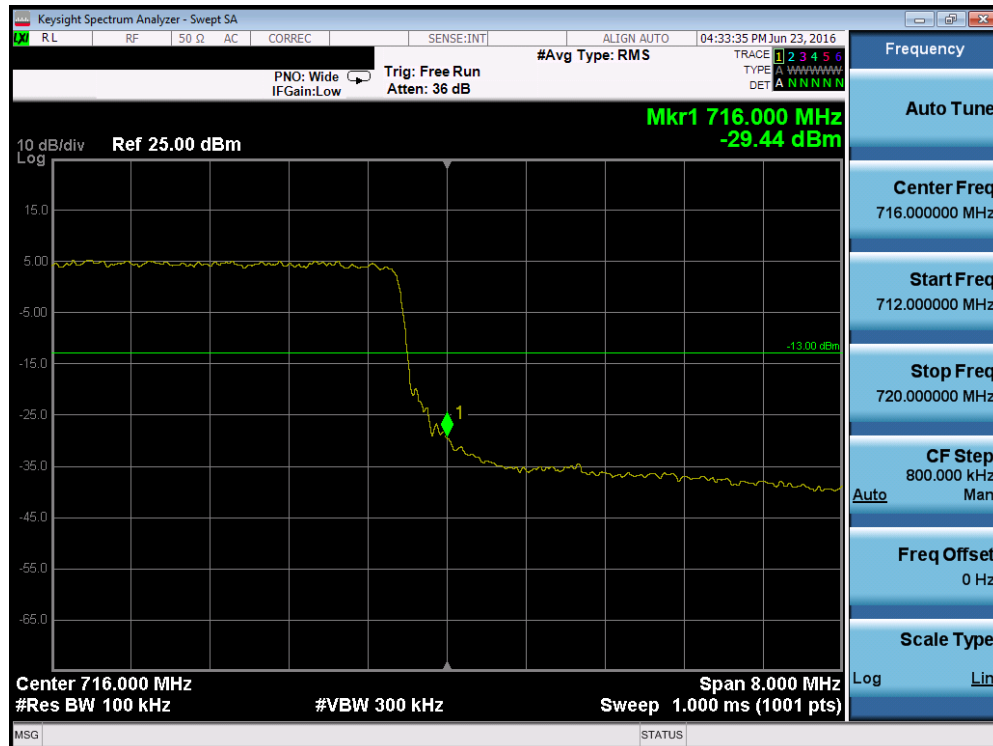
Plot 7-92. Upper Band Edge Plot (Band 12 – 10.0MHz QPSK – RB Size 50)
