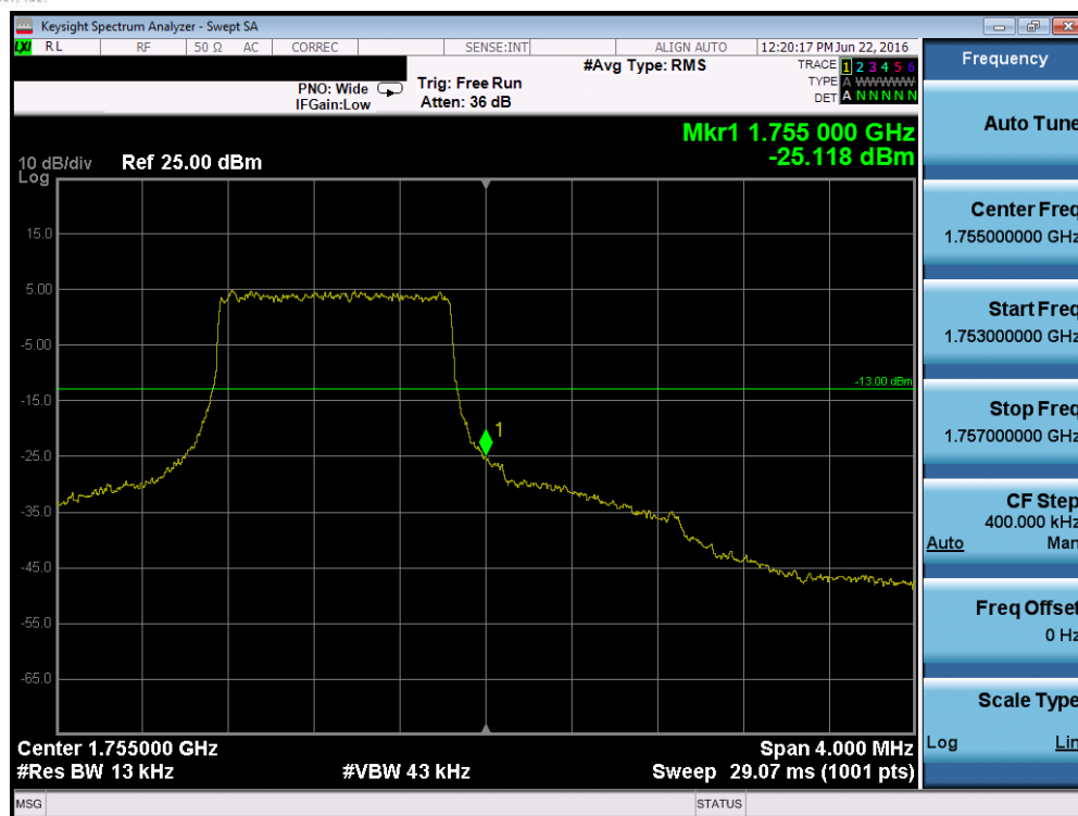
Plot 7-111. Upper Band Edge Plot (Band 4 – 1.4MHz QPSK – RB Size 6)
