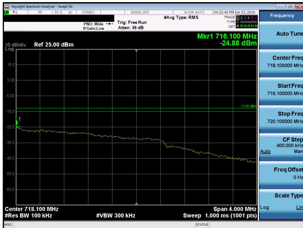
Plot 7-86. Upper Extended Band Edge Plot (Band 12 – 3.0MHz QPSK – RB Size 15)
