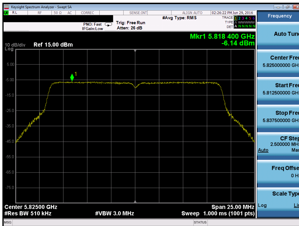
Plot 7-71. Power Spectral Density Plot (20MHz BW 802.11n (UNII Band 3) – Ch. 165)
