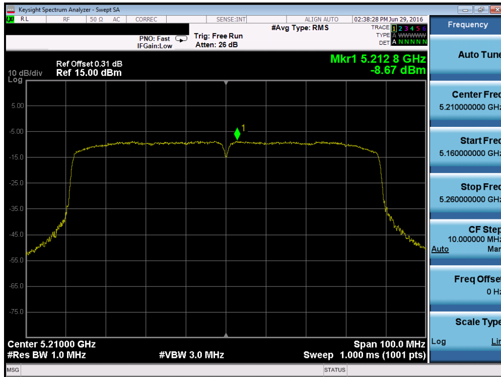
Plot 7-46. Power Spectral Density Plot (80MHz BW 802.11ac (UNII Band 1) – Ch. 42)
