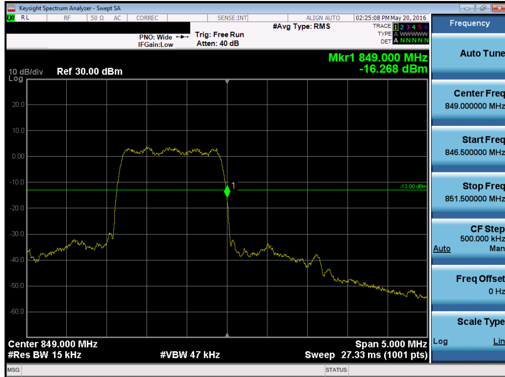
Plot 7-81. Band Edge Plot (Cellular CDMA Mode – Ch. 777)
