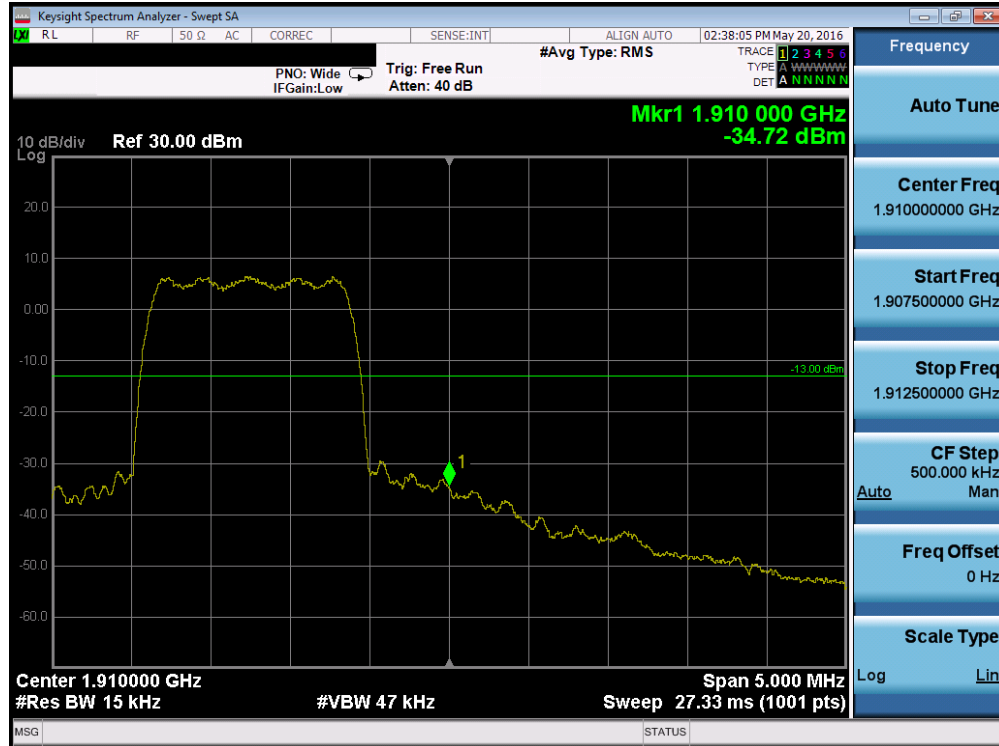
Plot 7-85. Band Edge Plot (PCS CDMA Mode – Ch. 1175)
