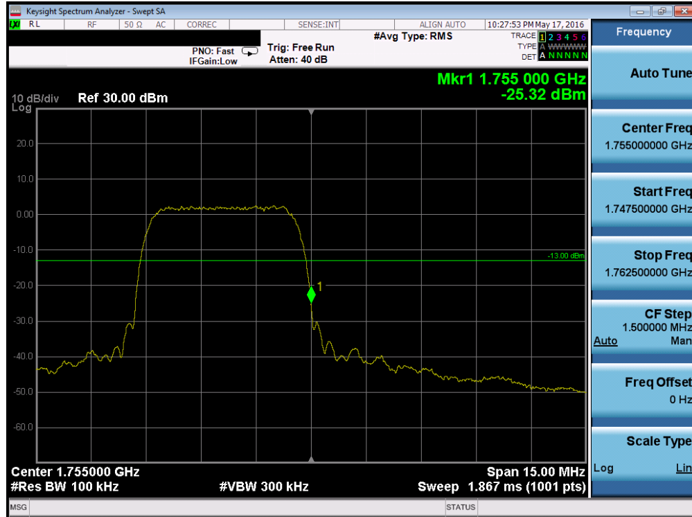
Plot 7-91. Band Edge Plot (AWS WCDMA Mode – Ch. 1862)
