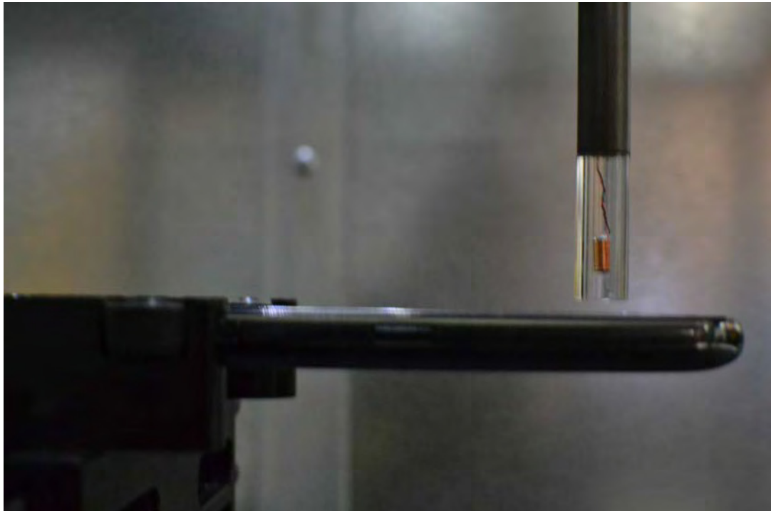
Figure 13-2 Test Setup for Wireless Device
