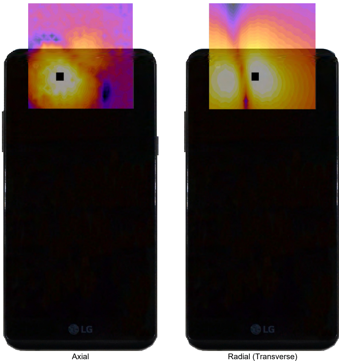
Figure 13-3 T-Coil Scan Overlay Magnetic Field Distributions
