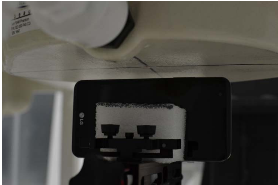
SAR Test Setup Photo 10 – Left at 10mm
