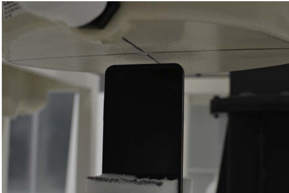
SAR Test Setup Photo 8 – Top at 10 mm
