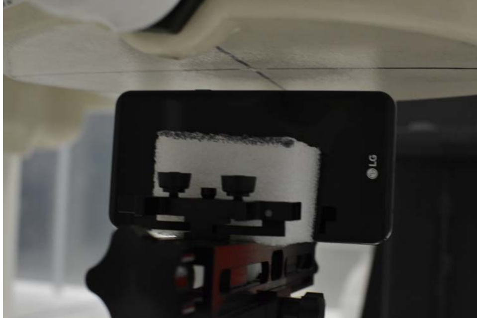
SAR Test Setup Photo 9 - Right at 10mm
