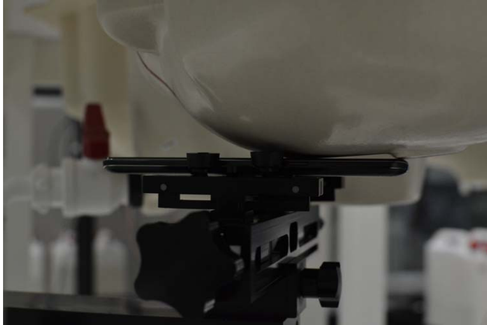
SAR Test Setup Photo 3 – Left Cheek
