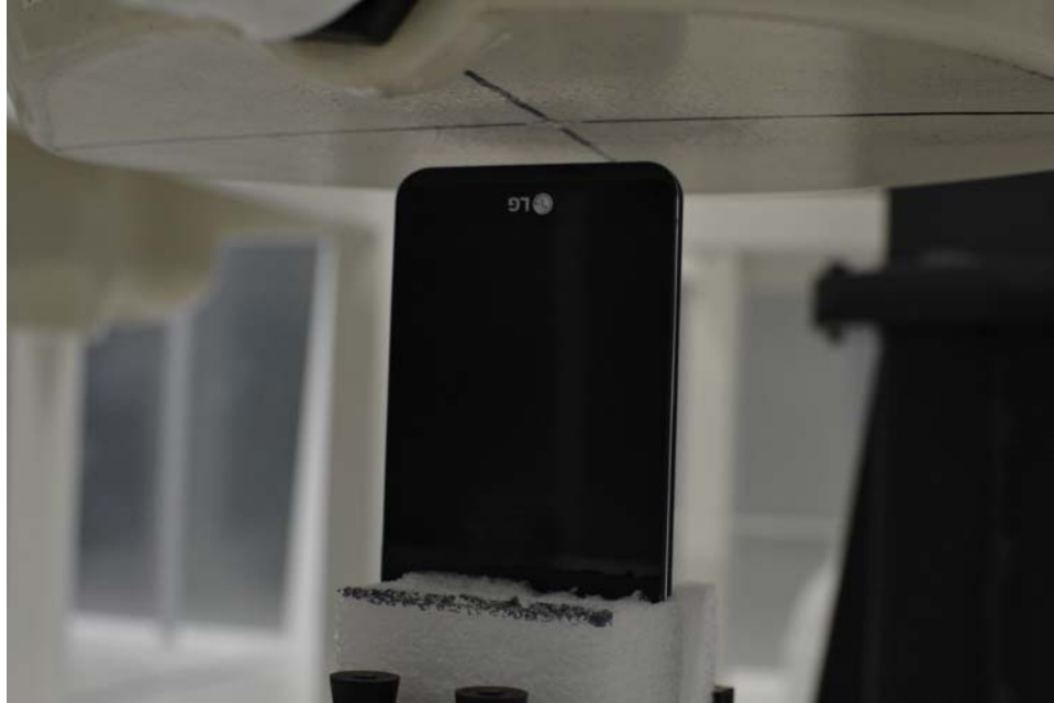
SAR Test Setup Photo 7 – Bottom at 10mm
