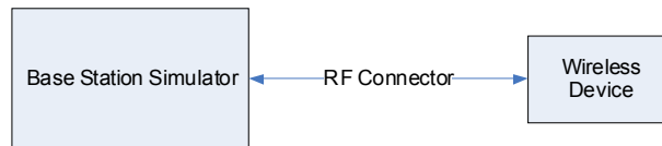
Figure 9-3 Power Measurement Setup
