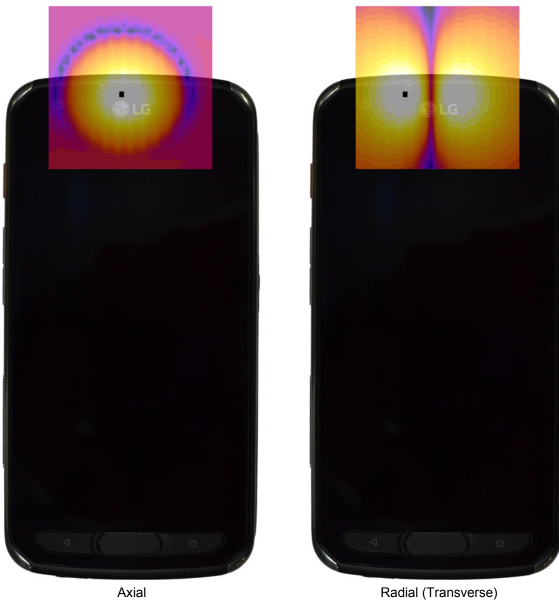
Figure 13-3 T-Coil Scan Overlay Magnetic Field Distributions
