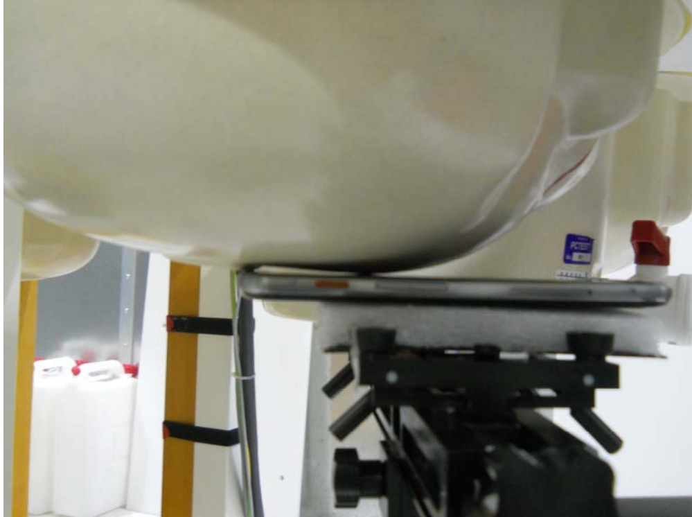
SAR Test Setup Photo 1: Right Cheek
