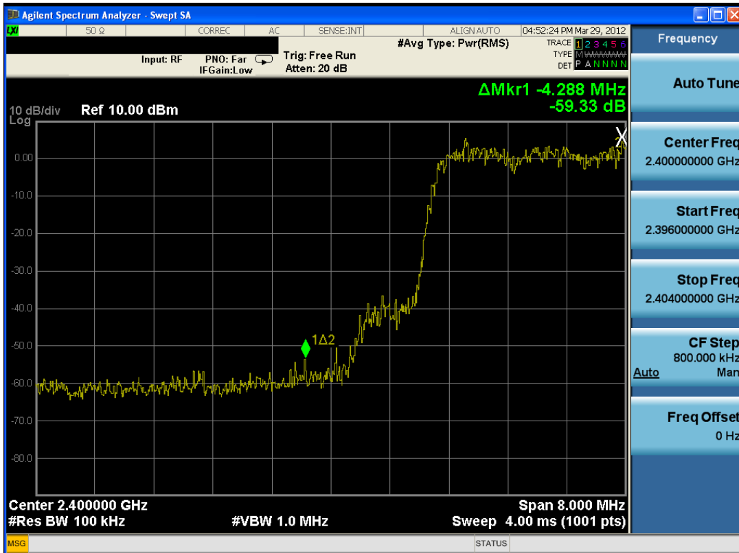
Plot 6-12. Band Edge Plot (Bluetooth with Hopping Enabled, 3Mbps – Ch. 0)
