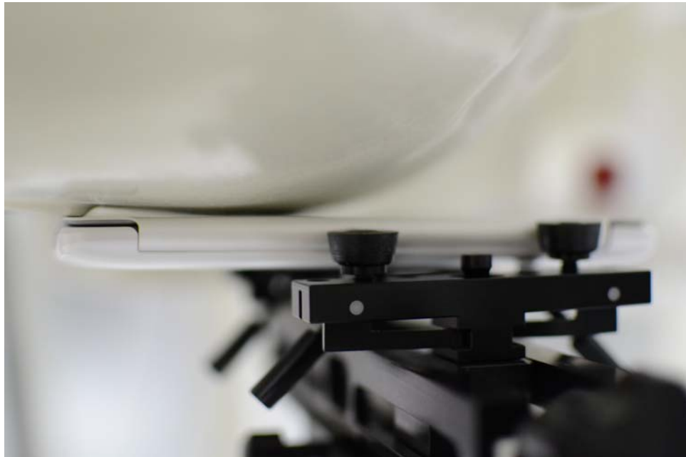
SAR Test Setup Photo 2: Right Cheek with Wireless Charging Cover Closed
