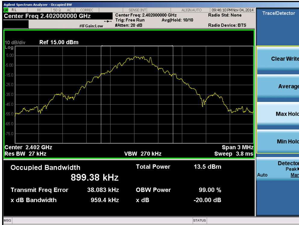
Plot 6-1. 20dB Bandwidth Plot (Bluetooth, 1Mbps – Ch. 0)
