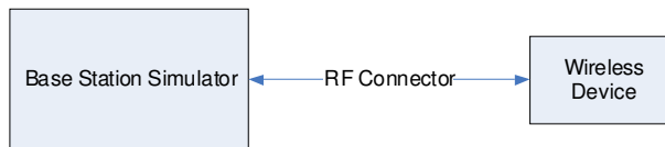
Figure 9-2 Power Measurement Setup
