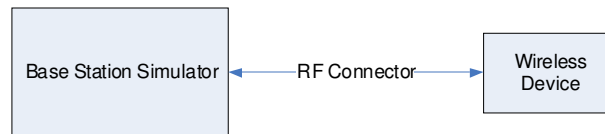
Figure 9-1 Power Measurement Setup
