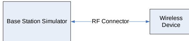
Figure 9-2 Power Measurement Setup
