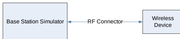
Figure 9-3 Power Measurement Setup
