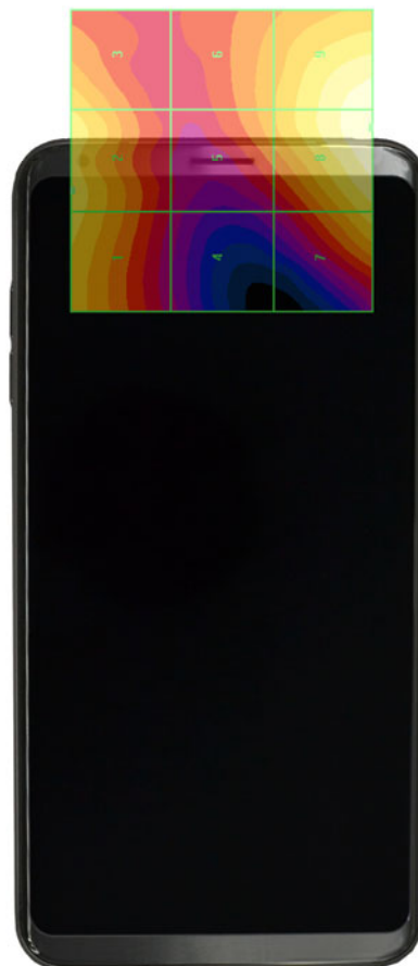
Figure 18-4 E-Field WD Scan overlay
