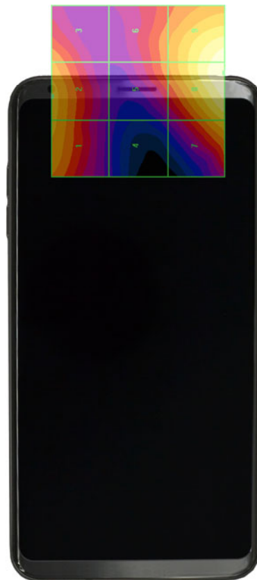
Figure 18-4 E-Field WD Scan overlay
