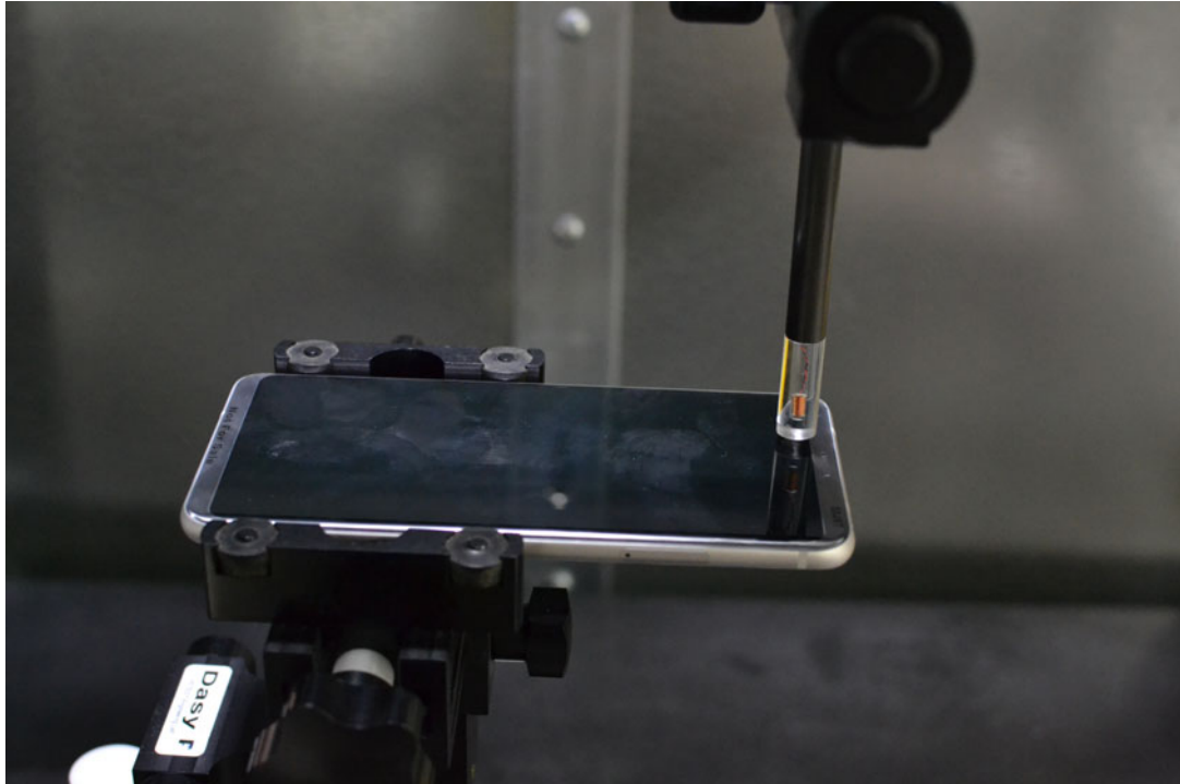
Figure 14-1 Test Setup for Wireless Device
