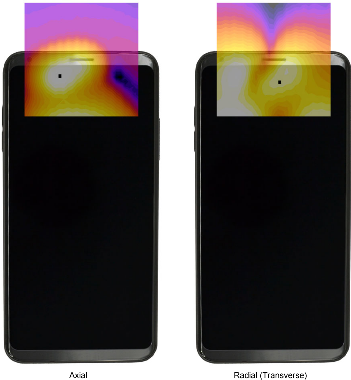
Figure 14-3 T-Coil Scan Overlay Magnetic Field Distributions
