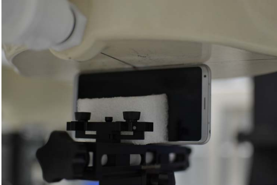
SAR Test Setup Photo 15: Left at 0.0 cm
