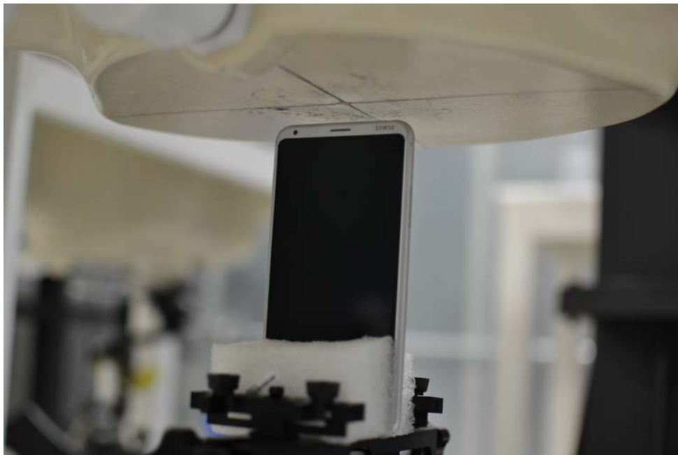
SAR Test Setup Photo 10: Top at 1.0 cm
