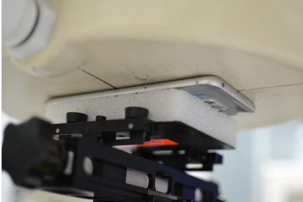
SAR Test Setup Photo 9: Front at 0.0 cm
