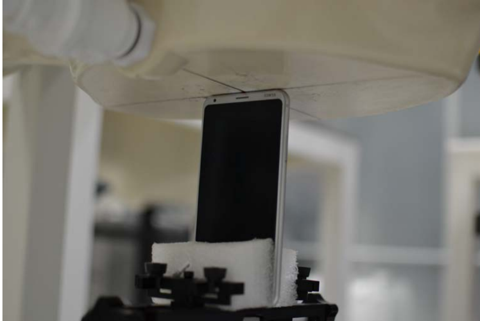
SAR Test Setup Photo 11: Top at 0.0 cm
