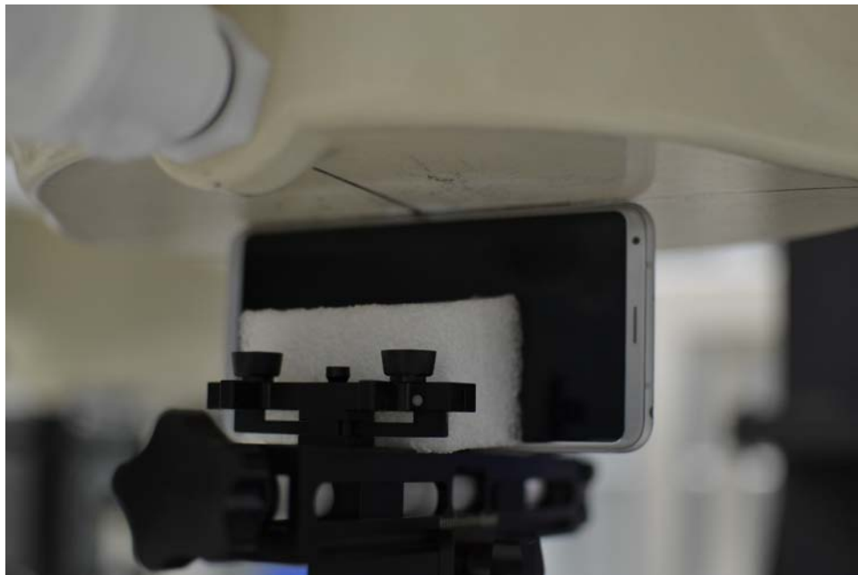
SAR Test Setup Photo 14: Left at 0.0 cm
