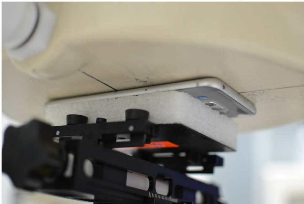
SAR Test Setup Photo 8: Front at 0.0 cm
