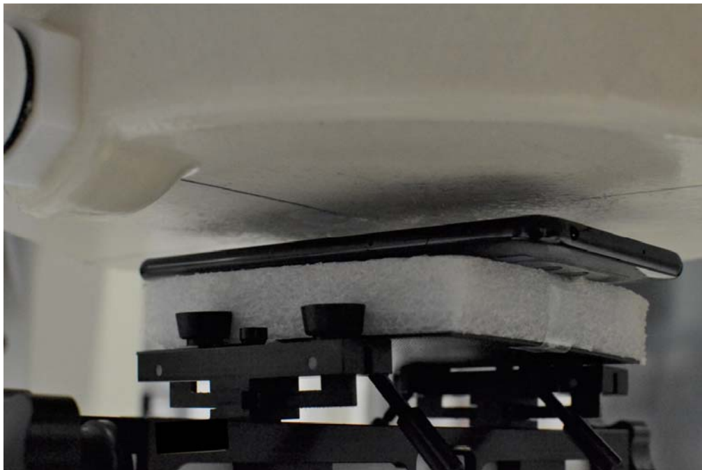
SAR Test Setup Photo 6: Front at 1.0cm
