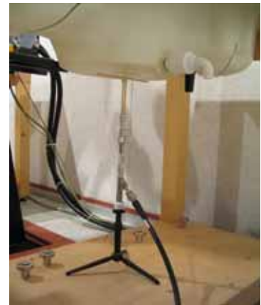
Photo of the dipole Antenna
