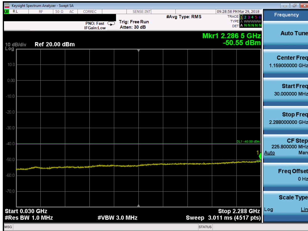
Plot 7-145. Conducted Spurious Plot (Band 30 - 5.0MHz QPSK - RB Size 1, RB Offset 0 - High Channel)
