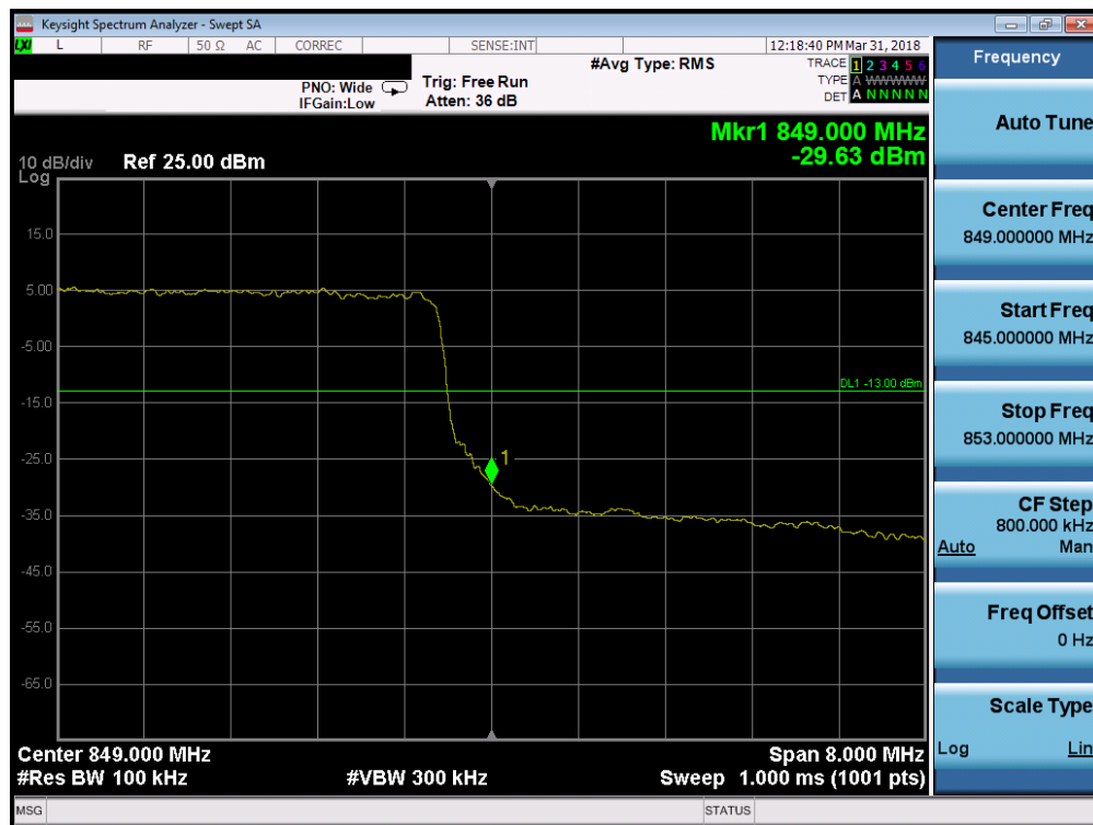
Plot 7-191. Upper Band Edge Plot (Band 26/5 - 10.0MHz QPSK - Full RB Configuration)
