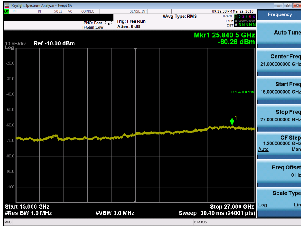
Plot 7-147. Conducted Spurious Plot (Band 30 - 5.0MHz QPSK - RB Size 1, RB Offset 0 - High Channel)
