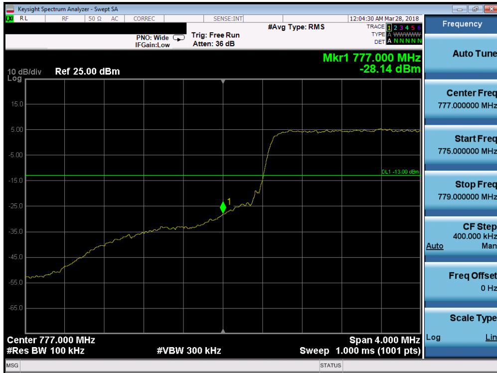
Plot 7-176. Lower Band Edge Plot (Band 13 - 5.0MHz QPSK - Full RB Configuration)
