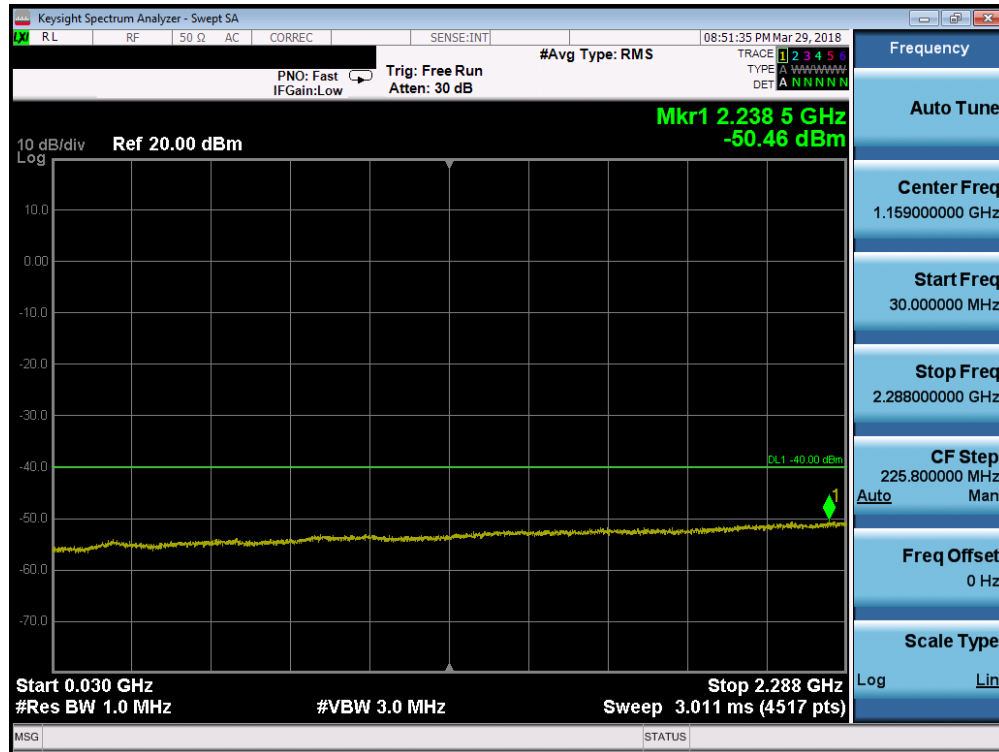
Plot 7-139. Conducted Spurious Plot (Band 30 - 5.0MHz QPSK - RB Size 1, RB Offset 0 - Low Channel)
