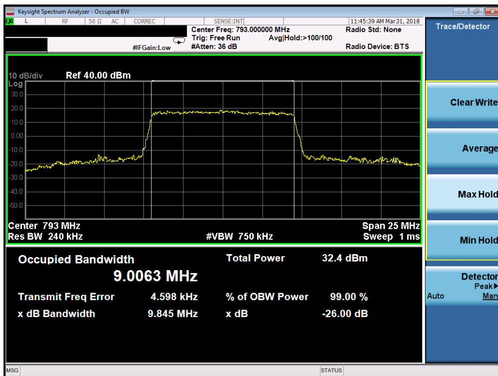
Plot 7-21. Occupied Bandwidth Plot (Band 14 - 10.0MHz 16-QAM - Full RB Configuration)
