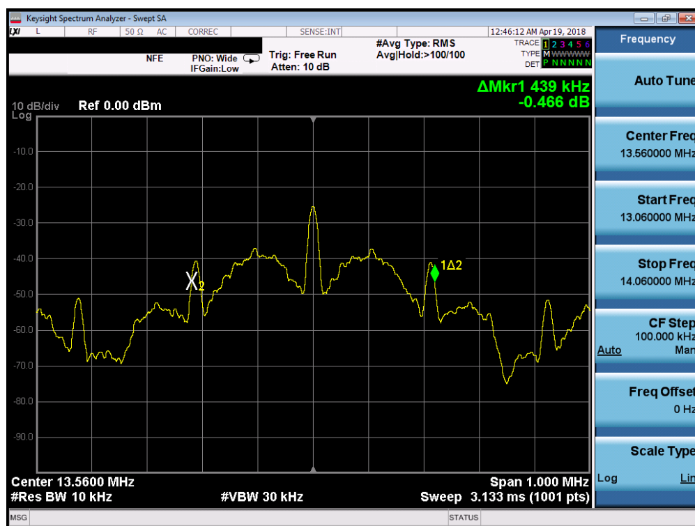
Figure 7-2. 20dB Bandwidth Plot
