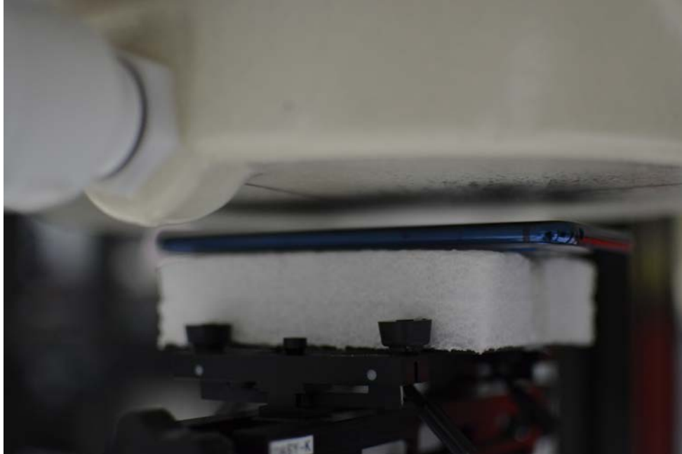
SAR Test Setup Photo 7: Front at 1.0 cm
