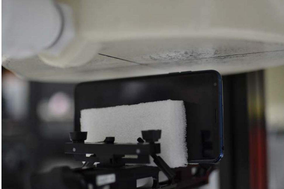
SAR Test Setup Photo 11: Left at 1.0 cm
