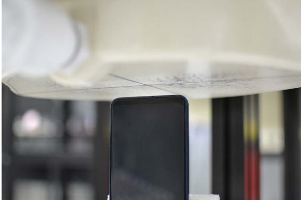
SAR Test Setup Photo 9: Bottom at 1.0 cm
