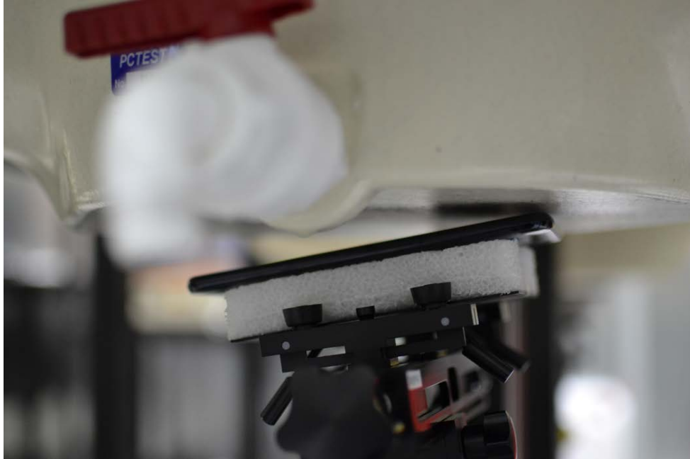
SAR Test Setup Photo 5: Mouth Jaw
