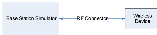
Figure 9-3 Power Measurement Setup
