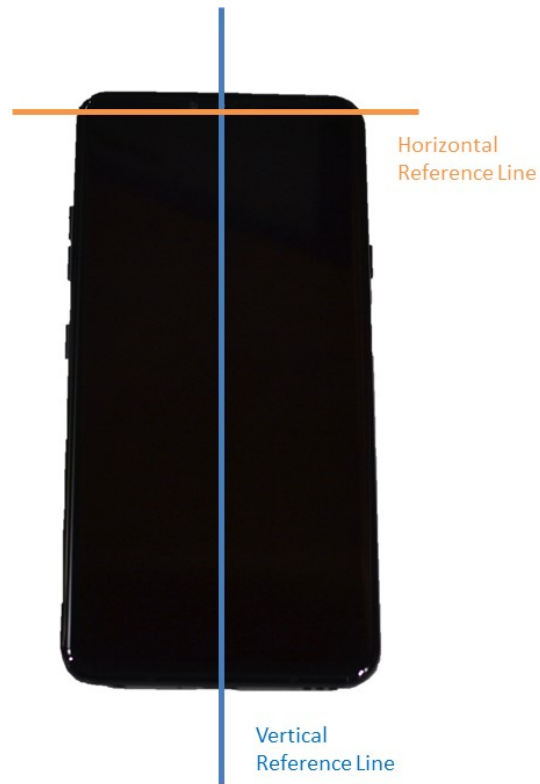
SAR Test Setup Photo 19 – Horizontal and Vertical Reference Lines
