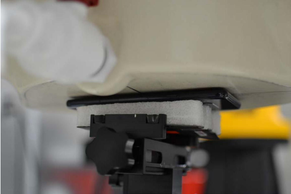
SAR Test Setup Photo 9 – Front Side at 2 mm
