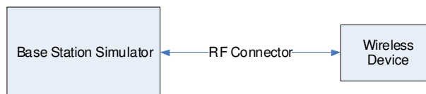
Figure 8-1 Power Measurement Setup
