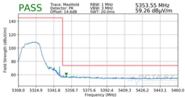
Plot 7-82. Radiated Upper Band Edge Plot MIMO (Peak – UNII Band 2A)
