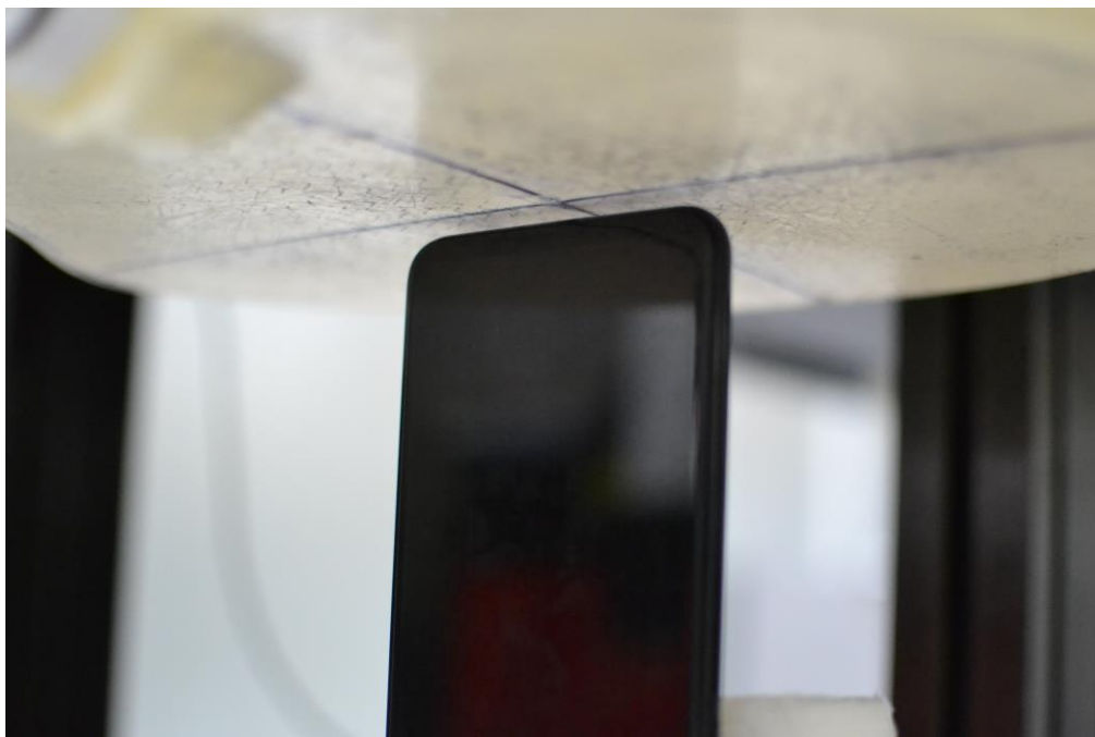
SAR Test Setup Photo 12 – Bottom Edge at 3mm
