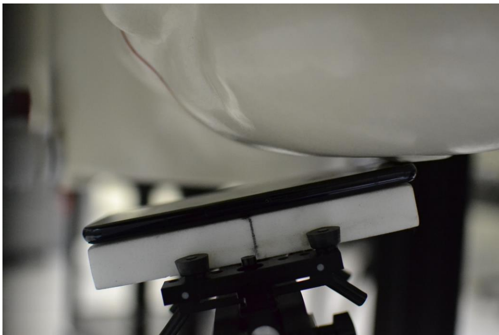
SAR Test Setup Photo 4 – Left Tilt
