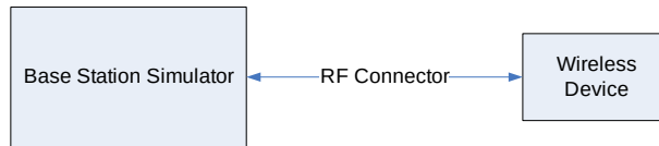
Figure 9-2 Power Measurement Setup
