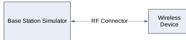
Figure 9-3 Power Measurement Setup
