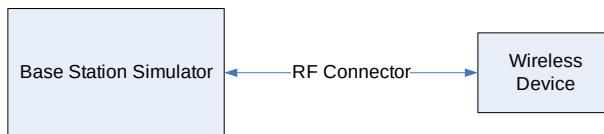
Figure 9-2 Power Measurement Setup
