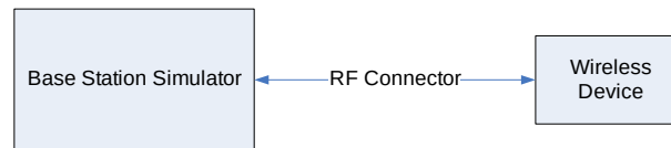
Figure 9-3 Power Measurement Setup
