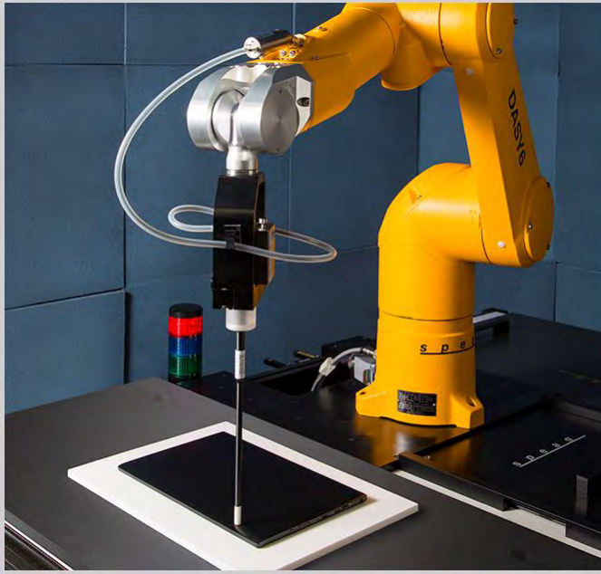
Figure A-1 Power density measurement system
