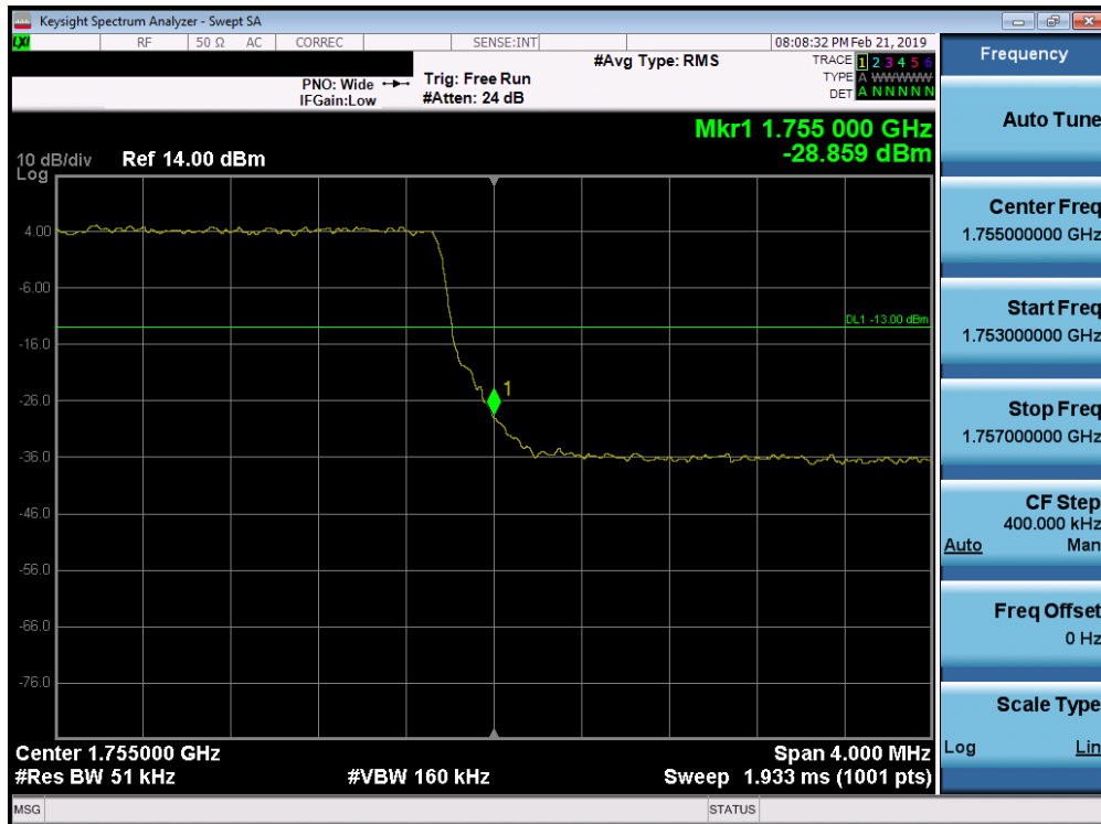
Plot 7-115. Upper Band Edge Plot (Band 4 - 5.0MHz QPSK - Full RB Configuration)
