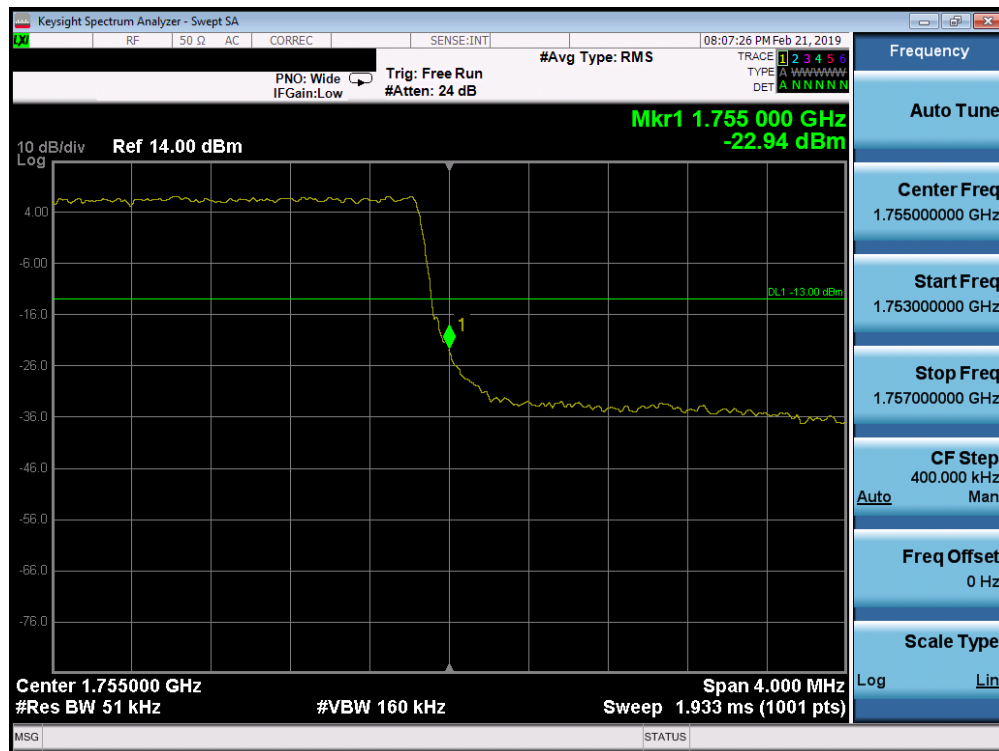
Plot 7-109. Upper Band Edge Plot (Band 4 - 3.0MHz QPSK - Full RB Configuration)
