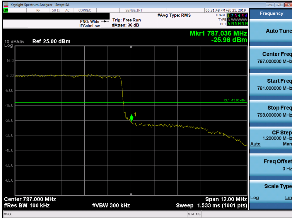
Plot 7-91. Upper Band Edge Plot (Band 13 - 10.0MHz QPSK - Full RB Configuration)
