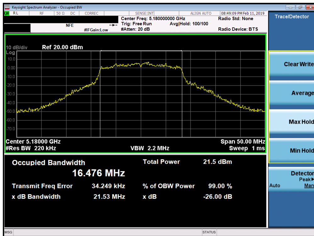
Plot 7-31. 26dB Bandwidth Plot SISO ANT2 (802.11a (UNII Band 1) – Ch. 36)
