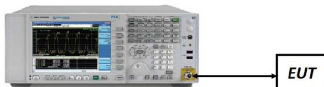
Figure 7-2. Test Instrument & Measurement Setup
