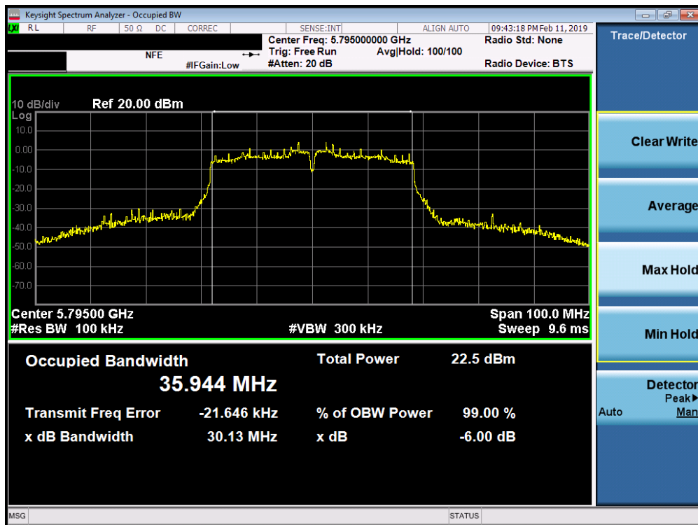
Plot 7-77. 6dB Bandwidth Plot SISO ANT2 (40MHz BW 802.11n (UNII Band 3) – Ch. 159)
