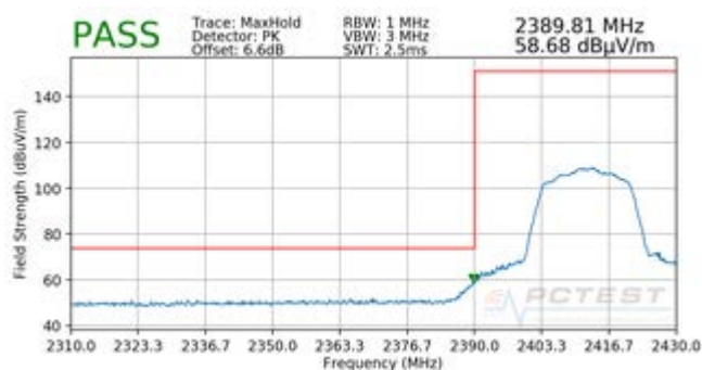
Plot 7-32. Radiated Restricted Lower Band Edge Measurement SDM (Peak)
