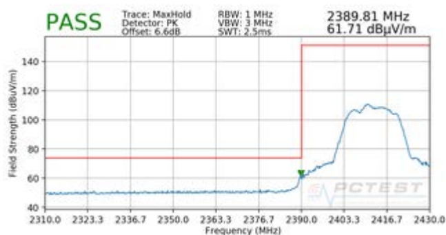
Plot 7-26. Radiated Restricted Lower Band Edge Measurement CDD (Peak)
