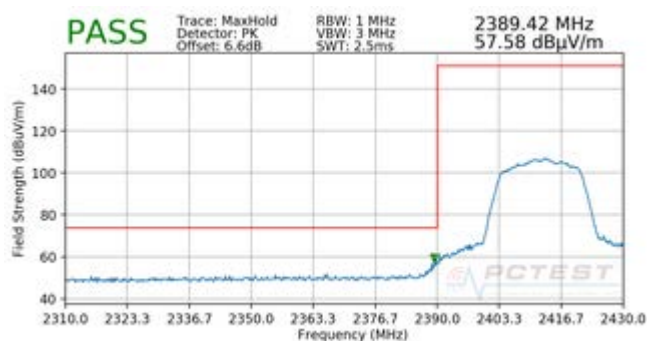
Plot 7-20. Radiated Restricted Lower Band Edge Measurement SISO ANT2 (Peak)
