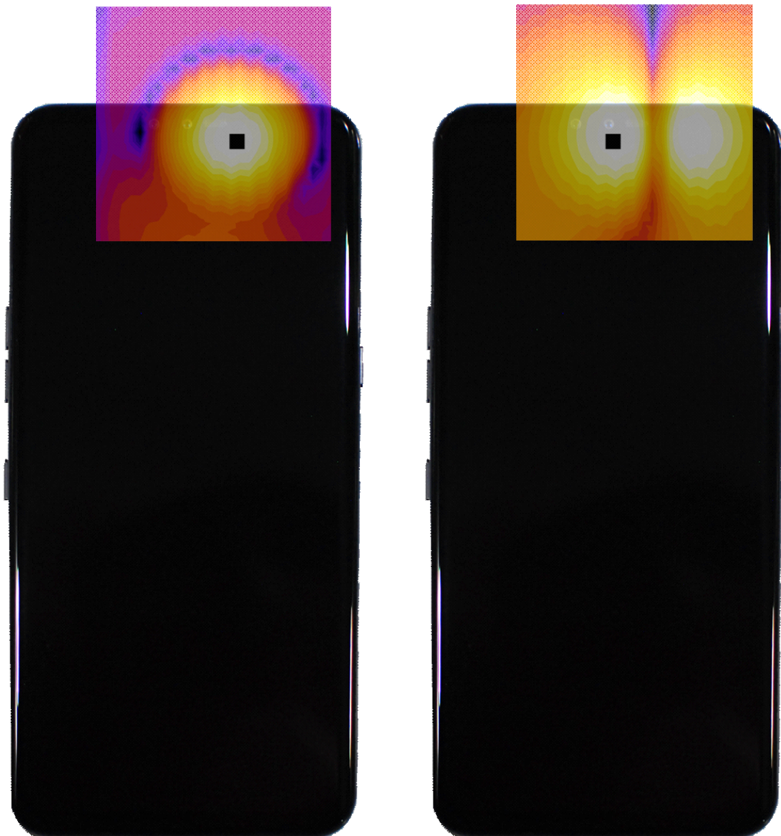
Figure 16-3 T-Coil Scan Overlay Magnetic Field Distributions
