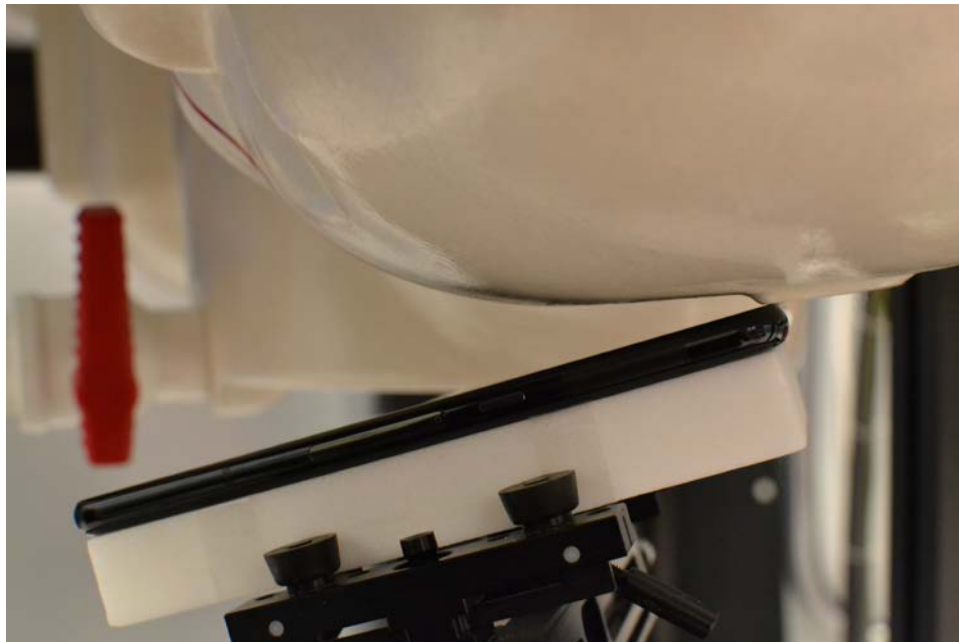
SAR Test Setup Photo 4 – Left Tilt
