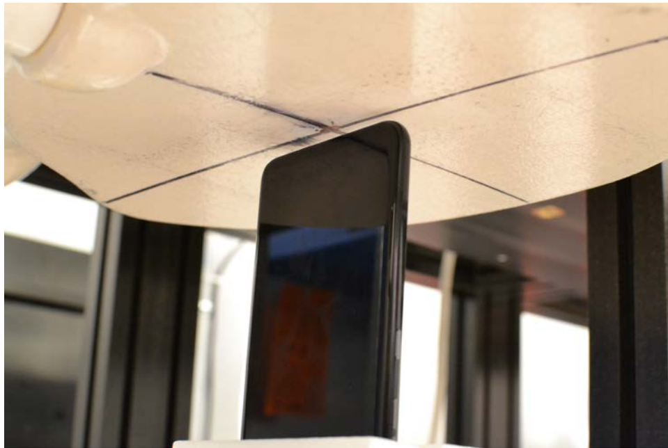
SAR Test Setup Photo 14 – Bottom Side at 3 mm
