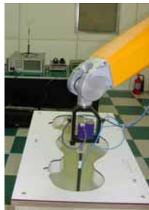
Figure 5. Photograph of the probe and the Phantom
