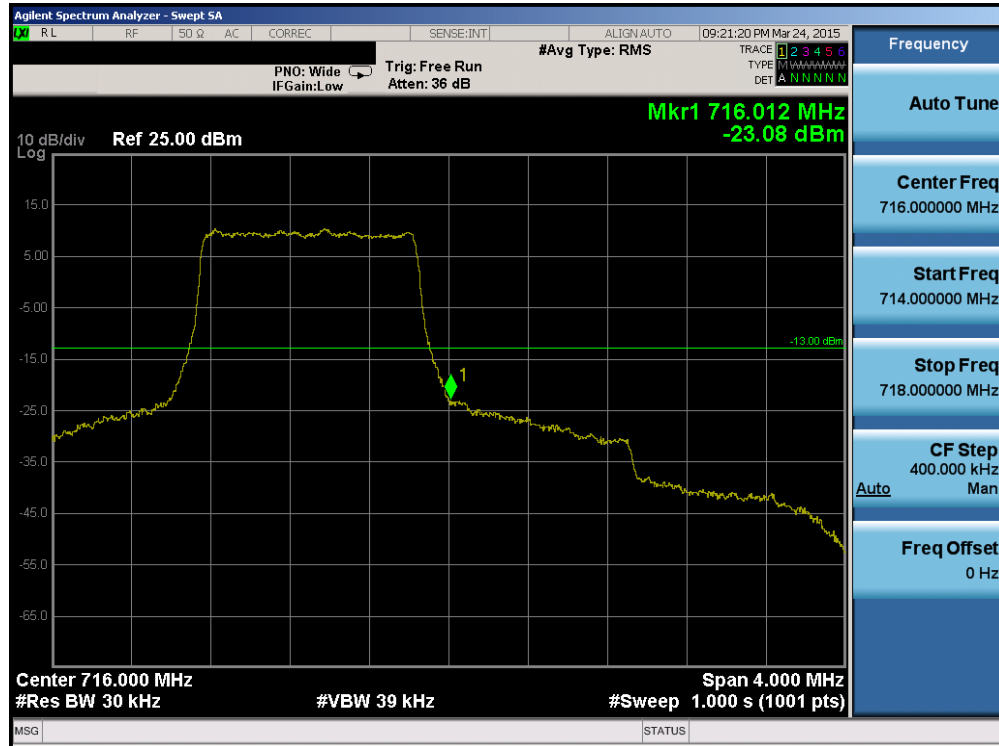
Plot 6-62. Upper Band Edge Plot (Band 12 – 1.4MHz QPSK – RB Size 6)
