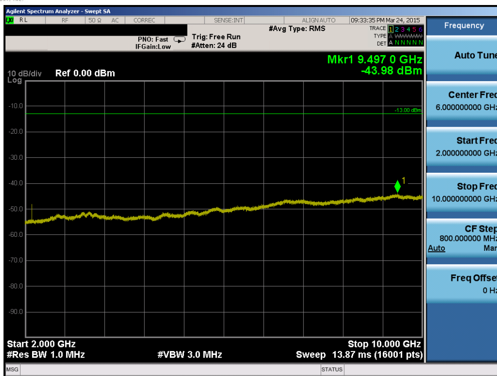
Plot 6-41. Conducted Spurious Plot (Band 12 – 3.0MHz QPSK – RB Size 1, RB Offset 0 – High Channel)
