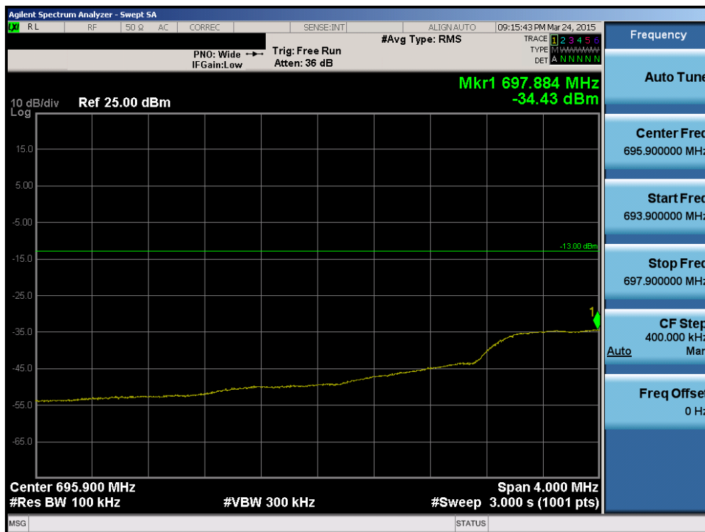
Plot 6-61. Lower Extended Band Edge Plot (Band 12 – 1.4MHz QPSK – RB Size 6)
