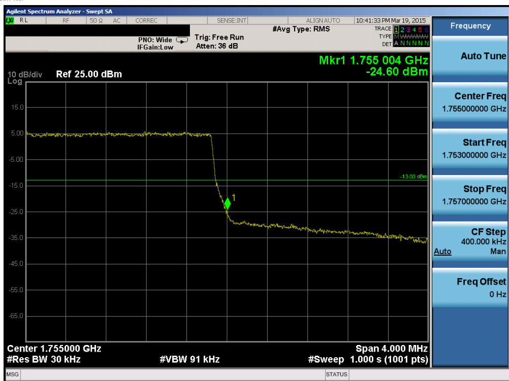
Plot 6-82. Upper Band Edge Plot (Band 4 – 3.0MHz QPSK – RB Size 15)
