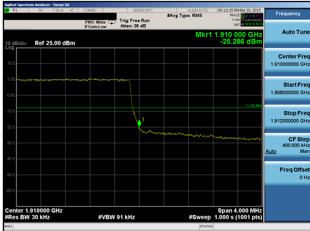
Plot 6-106. Upper Band Edge Plot (Band 2 – 3.0MHz QPSK – RB Size 15)
