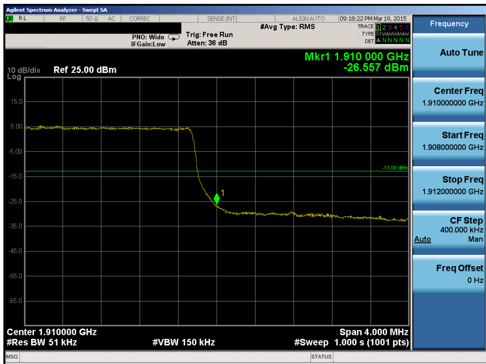
Plot 6-110. Upper Band Edge Plot (Band 2 – 5.0MHz QPSK – RB Size 25)
