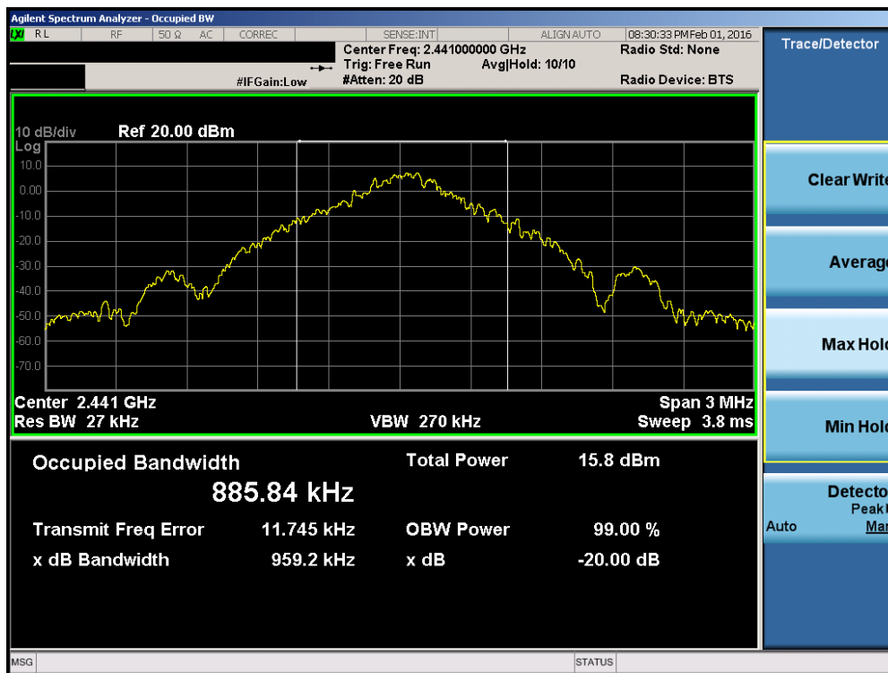
Plot 7-2. 20dB Bandwidth Plot (Bluetooth, 1Mbps – Ch. 39)
