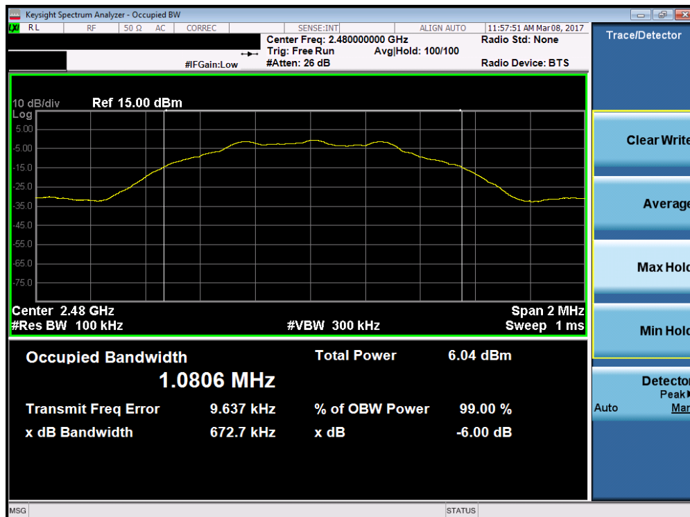
Plot 7-3. 6dB Bandwidth Plot (Bluetooth (LE) – Ch. 39)
