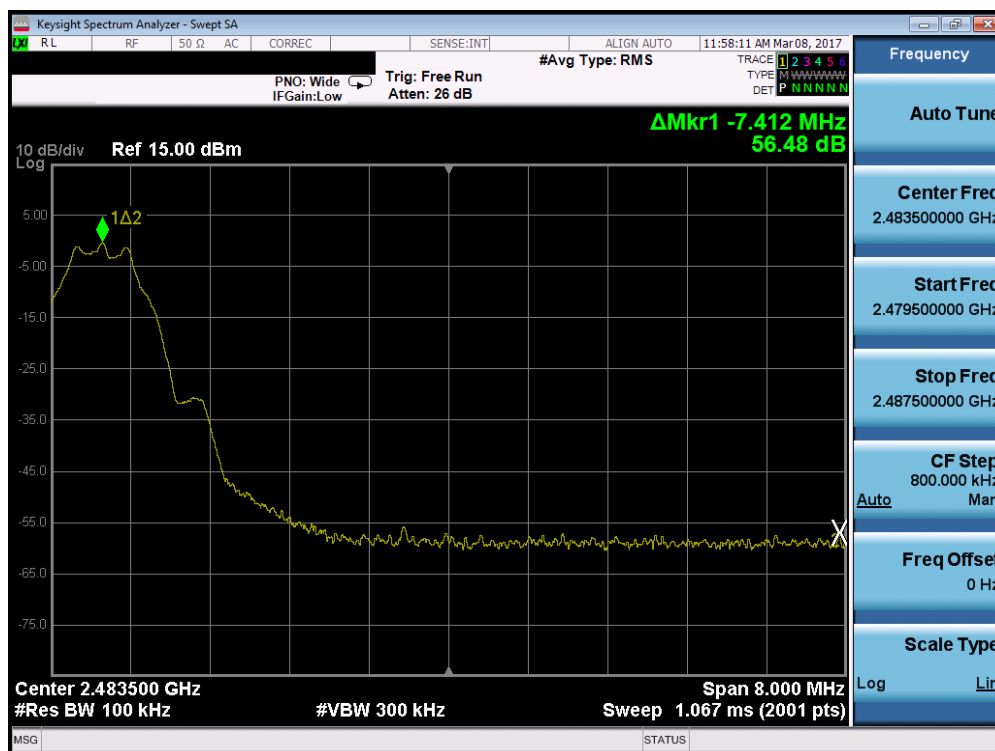
Plot 7-11. Band Edge Plot (Bluetooth (LE) - Ch. 39)
