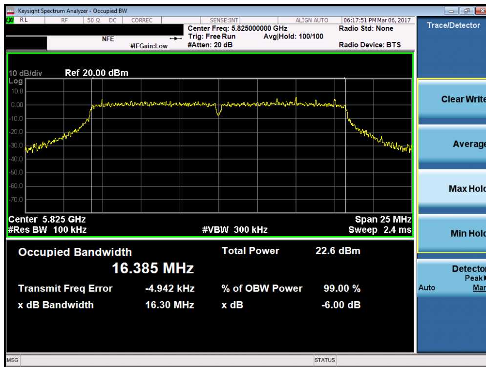
Plot 7-31. 6dB Bandwidth Plot (802.11a (UNII Band 3) – Ch. 165)
