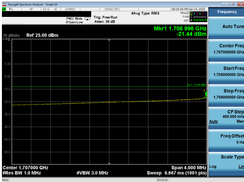
Plot 7-384. Lower Extended Band Edge Plot (Band n66 - 20.0MHz CP-OFDM-QPSK - Full RB Configuration)
