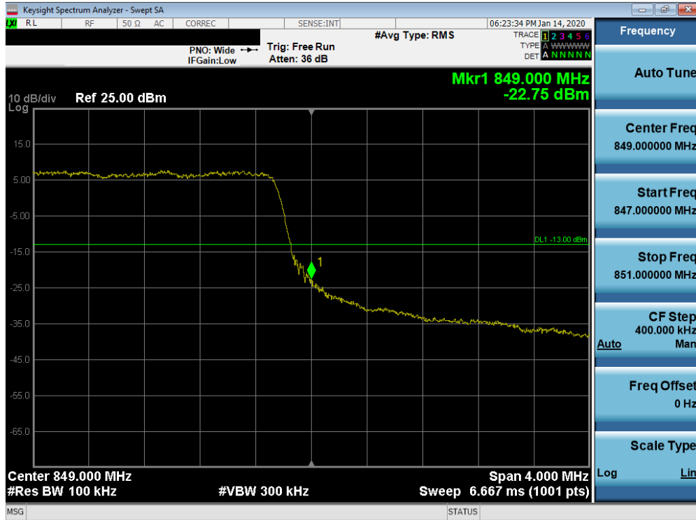
Plot 7-364. Upper Band Edge Plot (n5 - 5MHz DFT-s-OFDM-QPSK - Full RB Configuration)
