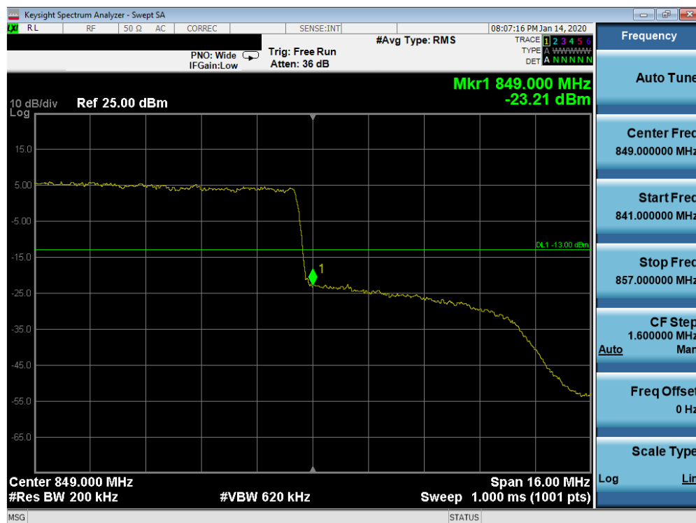
Plot 7-370. Upper Band Edge Plot (n5- 20MHz CP-OFDM-QPSK - Full RB Configuration)
