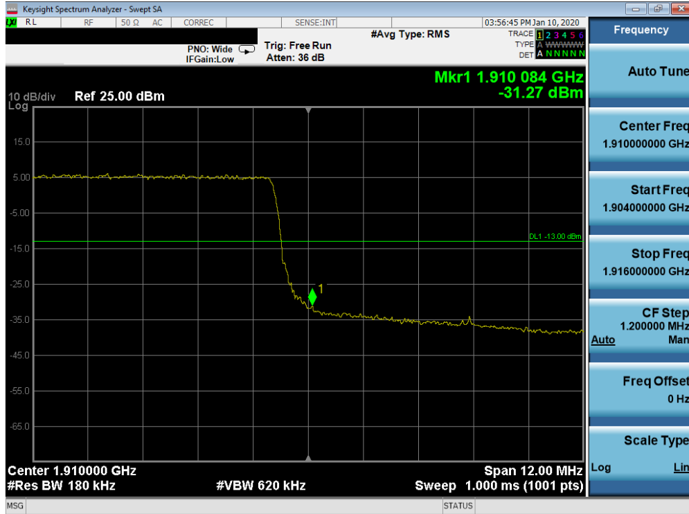
Plot 7-397. Upper Band Edge Plot (Band n2 - 15.0MHz CP-OFDM-QPSK - Full RB Configuration)
