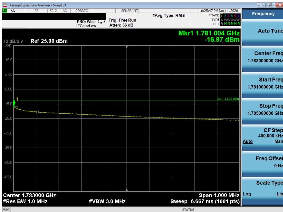
Plot 7-378. Upper Extended Band Edge Plot (Band n66 - 10.0MHz CP-OFDM-QPSK - Full RB Configuration)
