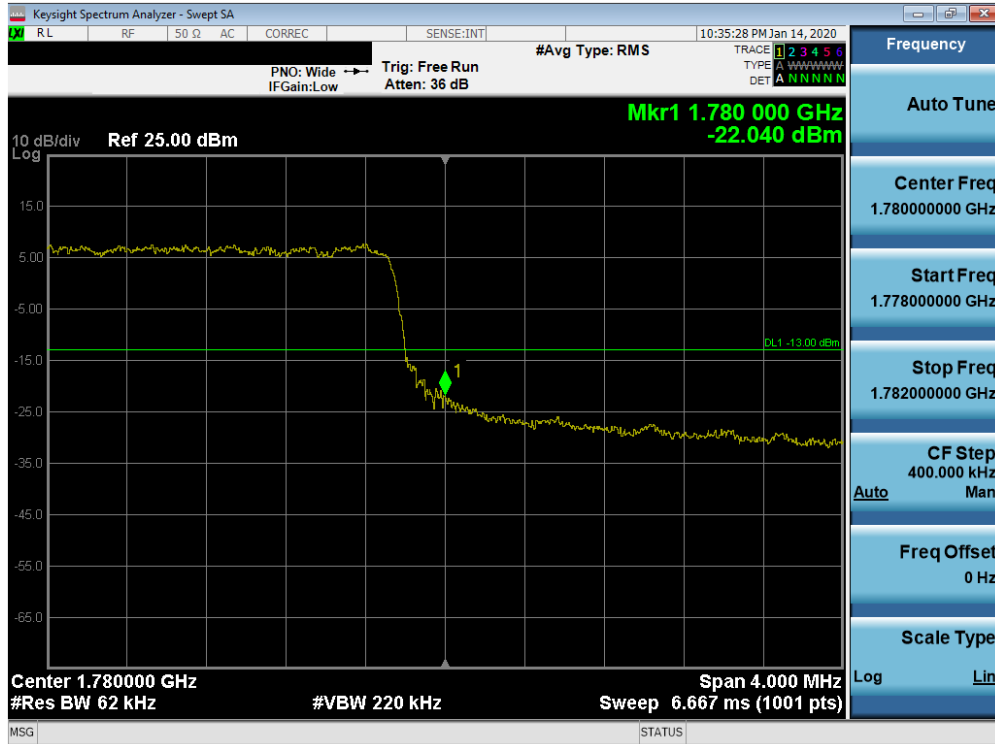
Plot 7-373. Upper Band Edge Plot (Band n66 - 5.0MHz CP-OFDM-QPSK - Full RB Configuration)
