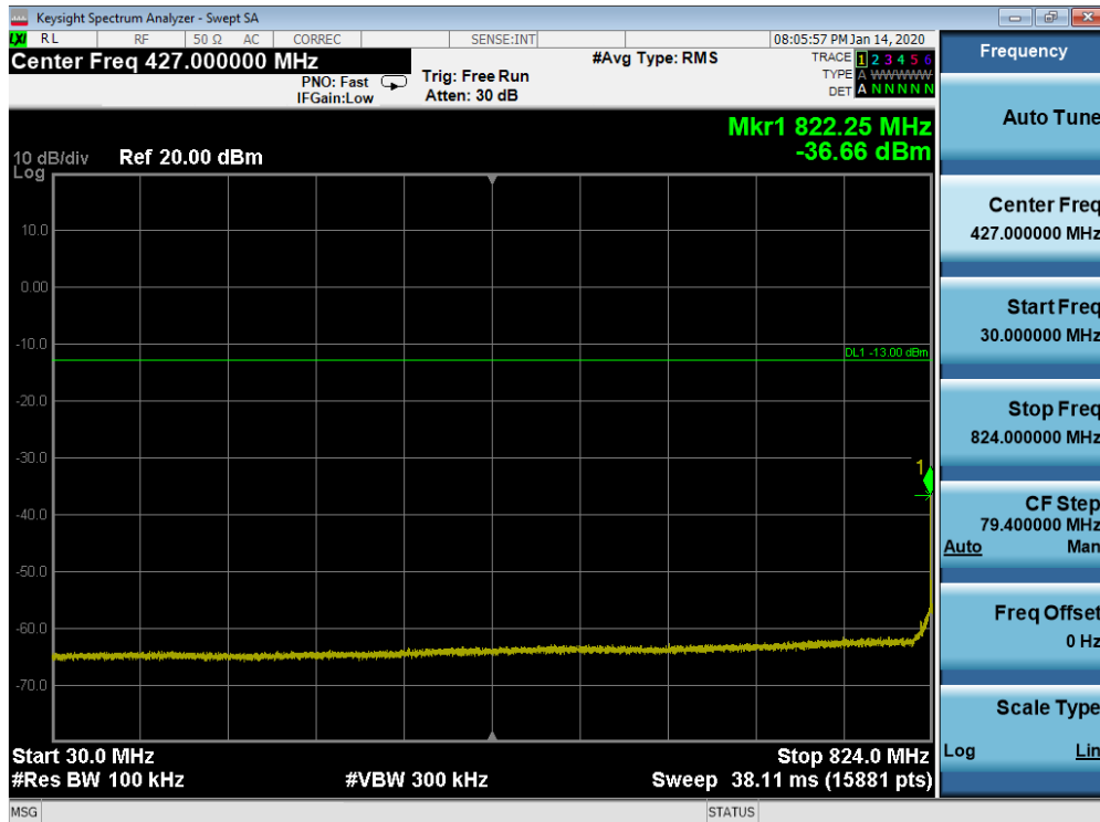
Plot 7-342. Conducted Spurious Plot (n5 - 5MHz DFT-s-OFDM-QPSK - RB Size 1, RB Offset 1 - High Channel)
