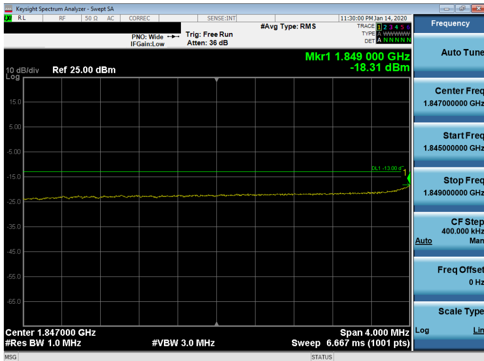
Plot 7-396. Lower Extended Band Edge Plot (Band n2 - 15.0MHz CP-OFDM-QPSK - Full RB Configuration)
