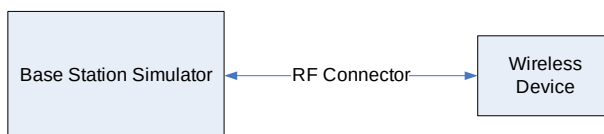
Figure 9-1 Power Measurement Setup
