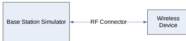
Figure 9-3 Power Measurement Setup
