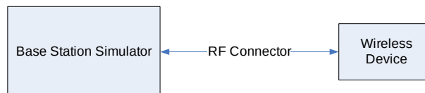
Figure 9-4 Power Measurement Setup
